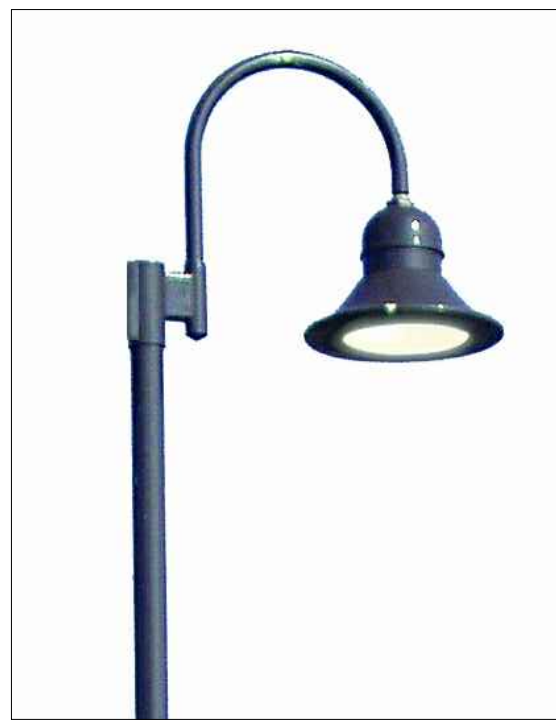
POLE MOUNTED LIGHT (L1) SELUX LIGHTING "BETA PENDANT" POLE MOUNTED 100W FIXTURE, MODEL RBPC-L-R2-1110-BK-100-HS-PC WITH LOW GLARE CUTOFF SHIELD, COLOR: BLACK PHOTOCELL CONTROL, OR APPROVED EQUAL. MOUNTING HEIGHT ON A35 SERIES BLACK ALUMINUM POLE = 12 FEET.
