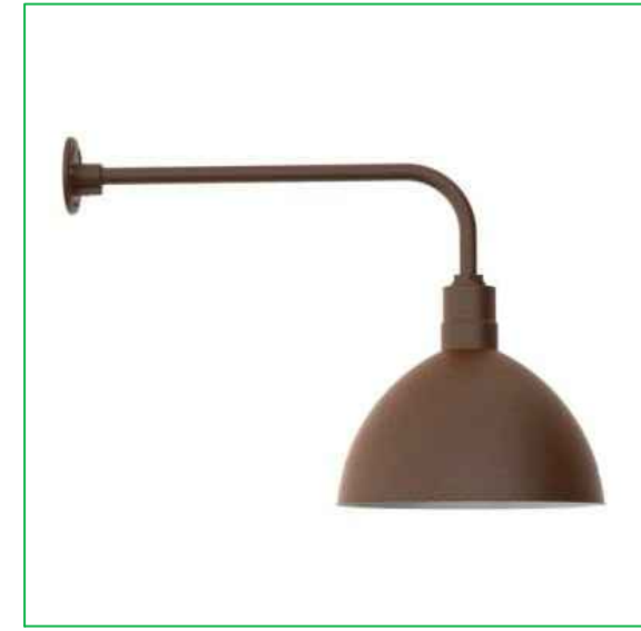
WALL MOUNTED HOUSE LIGHT (L2) BARNLIGHT ELECTRIC WALL MOUNTED FIXTURE, MODEL "WESCO GOOSENECK", 100W, COLOR: DARK GREEN METAL SHADE, OR APPROVED EQUAL. MOUNTING HEIGHT = 7 FEET.
