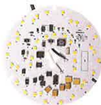
LED Light Engine (4" diameter)
