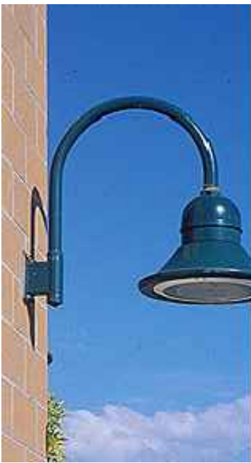
L2: Wall Mounted SELUX LIGHTING "BETA PENDANT" WALL MOUNTED FIXTURE. MODEL #BPC-L-R2-1-H50-BK-120-HS-PC WITH LOW GLARE CUTOFF SHIELD. COLOR: BLACK. PHOTOCCELL CONTROL. OR APPROVED EQUAL. MOUNTING HEIGHT = 10 FEET. DARK SKY COMPLIANT
