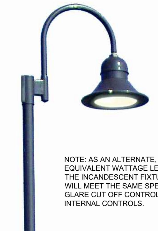
L3: Pole Mounted SELUX LIGHTING "BETA PENDANT" POLE MOUNTED 150W FIXTURE. MODEL #BPC-L-R2-1-H150-BK-120-HS-PC WITH LOW GLARE CUTOFF SHIELD, COLOR: BLACK. TIMER CONTROL OR APPROVED EQUAL MOUNTING HEIGHT ON A35 SERIES BLACK ALUMINUM POLE = 12 FEET. DARK SKY COMPLIANT
