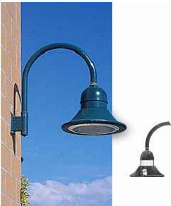
L2: Wall Mounted SELUX LIGHTING "BETA PENDANT" WALL MOUNTED FIXTURE. MODEL #BPC-L-R2-1-H50-BK-120-HS-PC WITH LOW GLARE CUTOFF SHIELD, COLOR: BLACK. PHOTOCELL CONTROL OR APPROVED EQUAL MOUNTING HEIGHT = 10 FEET DARK SKY COMPLIANT
