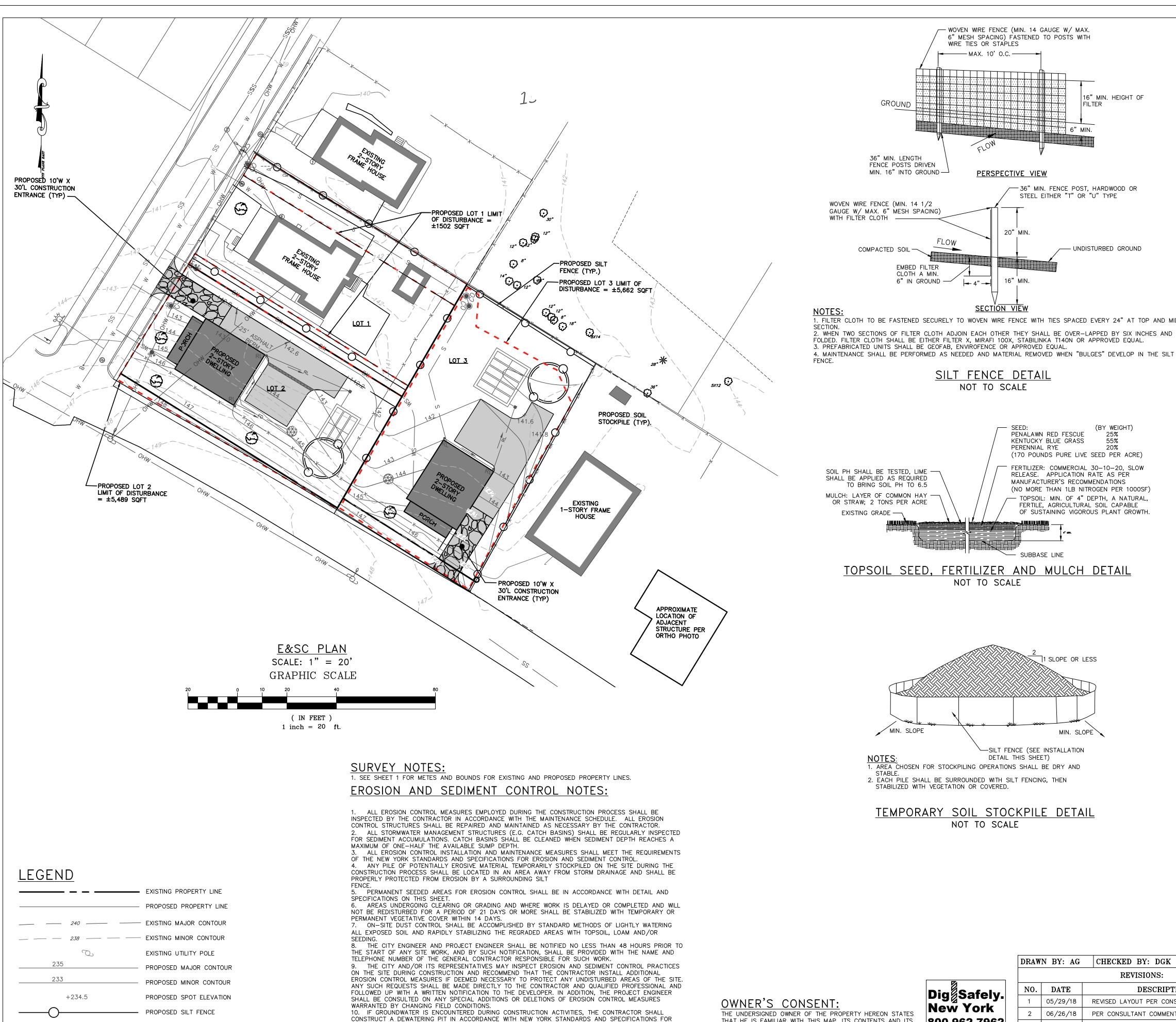
EROSION AND SEDIMENT CONTROL TO FILTER WATER FOR PUMPING TO A SUITABLE LOCATION.
