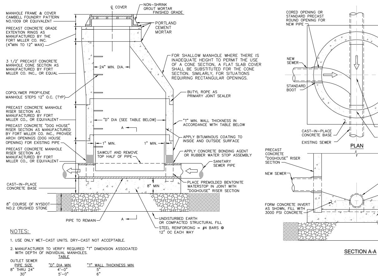
PRECAST CONCRETE INSERTION "DOGHOUSE" MANHOLE DETAIL NOT TO SCALE
