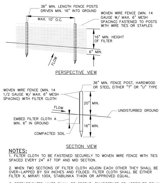
3. PREFABRICATED UNITS SHALL BE GEOFAB, ENVIROFENCE OR APPROVED EQUAL. 4. MAINTENANCE SHALL BE PERFORMED AS NEEDED AND MATERIAL REMOVED WHEN "BULGES" DEVELOP IN THE SILT FENCE.
