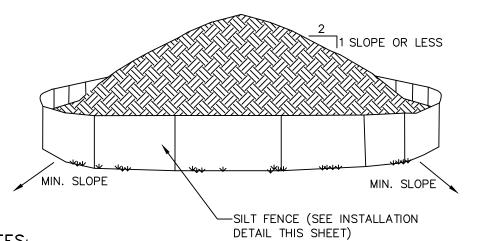
. AREA CHOSEN FOR STOCKPILING OPERATIONS SHALL BE DRY AND STABLE. 2. EACH PILE SHALL BE SURROUNDED WITH SILT FENCING, THEN STABILIZED WITH VEGETATION OR COVERED.
