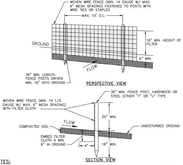
1. FILTER CLOTH TO BE FASTENED SECURELY TO WOVEN WIRE FENCE WITH TIES SPACED EVERY 24" AT TOP AND MID 2. WHEN TWO SECTIONS OF FILTER CLOTH ADJOIN EACH OTHER THEY SHALL BE OVER-LAPPED BY SIX INCHES AND FOLDED. FILTER CLOTH SHALL BE EITHER FILTER X, MIRAFI 100X, STABILINKA T140N OR APPROVED EQUAL. 3. PREFABRICATED UNITS SHALL BE GEOFAB, ENVIROFENCE OR APPROVED EQUAL. 4. MAINTENANCE SHALL BE PERFORMED AS NEEDED AND MATERIAL REMOVED WHEN "BULGES" DEVELOP IN THE SILT
