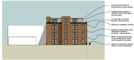
Elevation: Building 16: South Scale: 1/4" = 1'-0"
