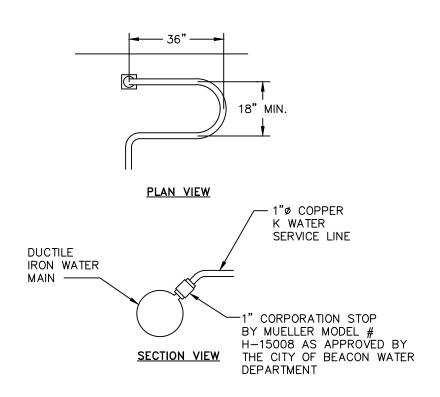
1. A MINIMUM 5' COVER SHALL BE PROVIDED ON THE WATER SERVICE LINE (CONDITIONED ON ACTUAL WATER MAIN DEPTH). 2. CORPORATION STOP TO BE COMPRESSION TYPE BY MUELLER. 3. WATER SERVICE LINE TO HAVE A 'GOOSENECK' NEAR CORPORATION 4. CORPORATION STOP TO BE INSTALLED IN THE UPPER HALF OF THE WATER MAIN AT AN ANGLE OF APPROXIMATELY 45° FROM
