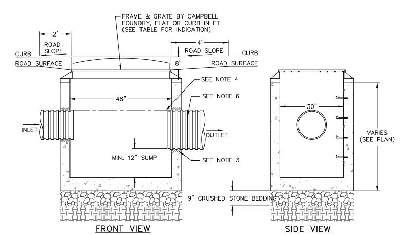
PRECAST CONCRETE CATCH BASIN WITH CONCRETE STRENGTH OF 4,000 PSI @ 28 DAYS.
