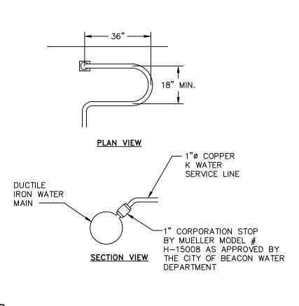
NOTES: 1. A MINIMUM 5' COVER SHALL BE PROVIDED ON THE WATER SERVICE LINE (CONDITIONED ON ACTUAL WATER MAIN DEPTH). 2. CORPORATION STOP TO BE COMPRESSION TYPE BY MUELLER. 3. WATER SERVICE LINE TO HAVE A 'GOOSENECK' NEAR CORPORATION STOP. 4. CORPORATION STOP TO BE INSTALLED IN THE UPPER HALF OF THE WATER MAIN AT AN ANGLE OF APPROXIMATELY 45' FROM HORIZONTAL.
