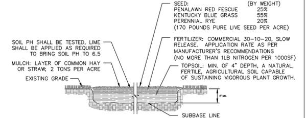
**TOPSOIL SEED, FERTILIZER AND MULCH DETAIL**
