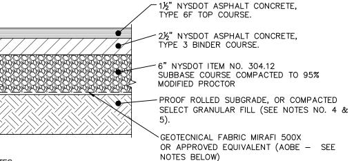
1. MATERIALS AND METHODS OF CONSTRUCTION SHALL BE IN CONFORMANCE WITH THE NEW YORK STATE DEPARTMENT OF TRANSPORTATION (NYSDOT) STANDARD SPECIFICATIONS FOR CONSTRUCTION AND MATERIALS, DATED JANUARY 2, 2002.
