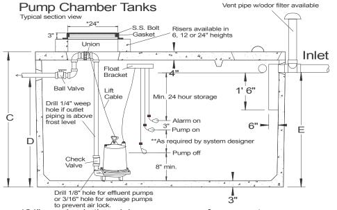
\*24" opening is the minimum necessary for access to a single pump. 30" opening for two pumps. Aluminum hatch doors are also available.
