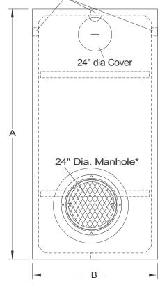
(3) 4" Polylok Inlets Baffle can be relocated to side inlet
