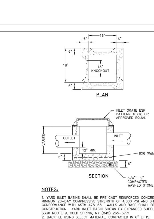
1. YARD INLET BASINS SHALL BE PRE CAST REINFORCED CONCRETE SHALL HAVE A MINIMUM 28-DAY COMPRESSIVE STRENGTH OF 4,000 PSI AND SHALL BE IN CONFORMANCE WITH ASTM 478-68. WALLS AND BASE SHALL BE ONE PIECE CONSTRUCTION. YARD INLET BASIN SHOWN BY EXPANDED SUPPLY PRODUCTS (ESP), 3330 ROUTE 9, COLD SPRING, NY (845) 265-3771.
