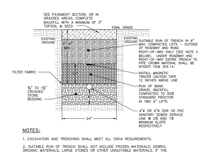
SANITARY SEWER SERVICE LINE TRENCH DETAIL
