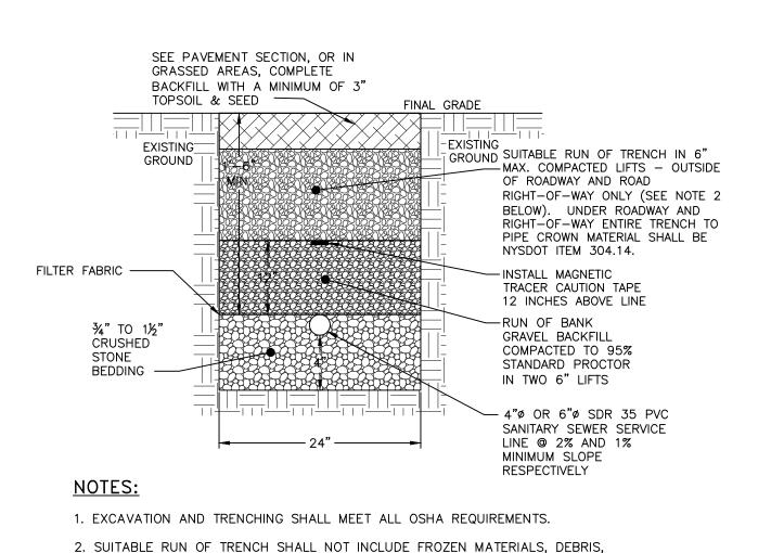
RUN OF TRENCH MATERIAL IS FOUND TO BE UNSUITABLE, A SUITABLE BACKFILL MATERIAL SHALL BE IMPORTED AND USED. SANITARY SEWER SERVICE LINE TRENCH DETAIL
