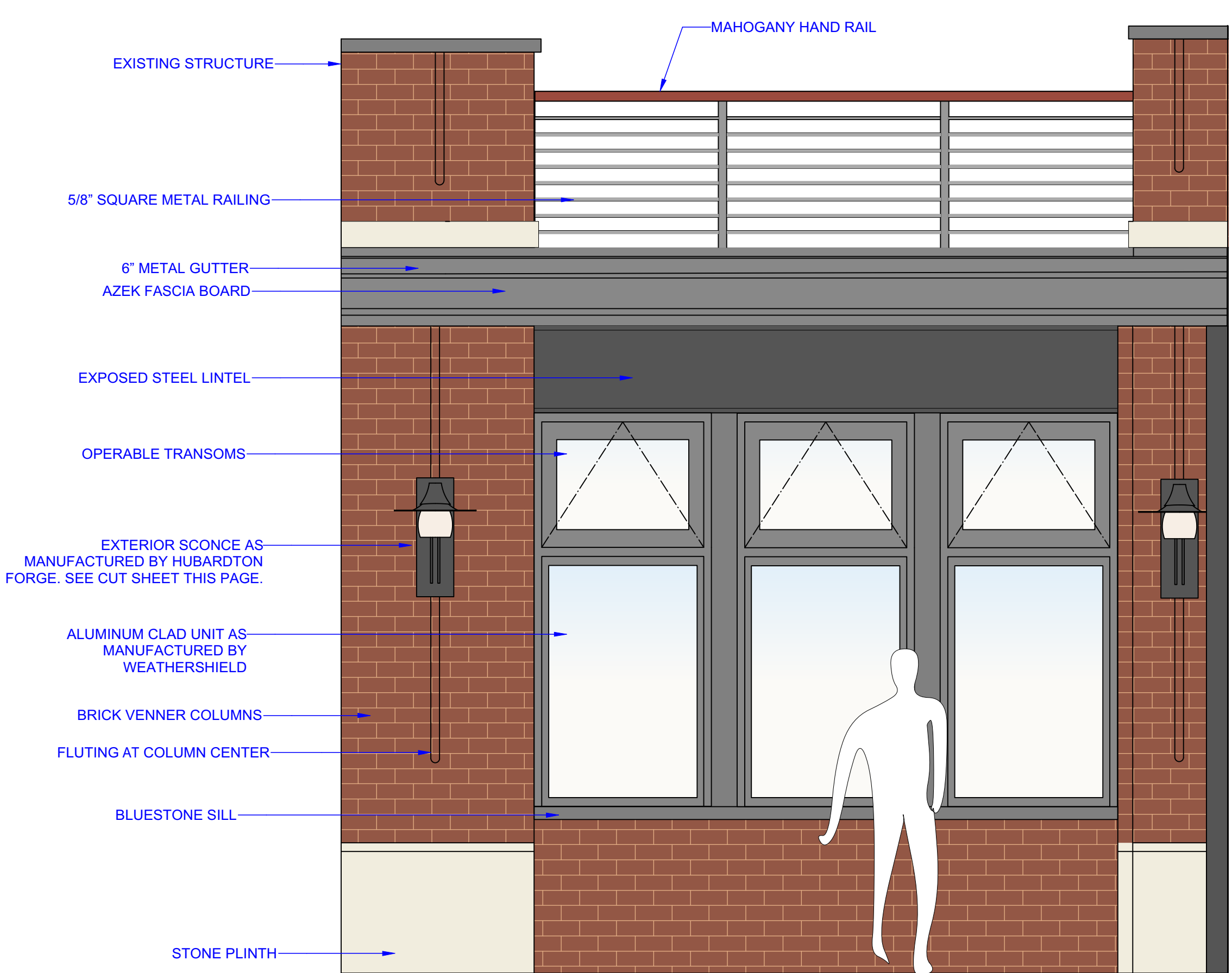
D-1 TYPICAL BAY DETAIL SCALE: 1/2"=1'-0"
