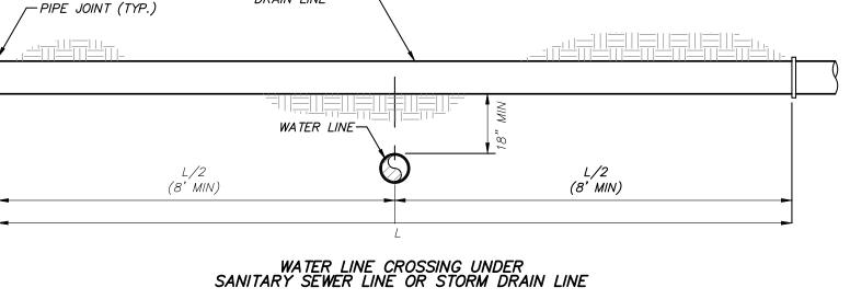
2. PROVIDE PIPE AND FITTING RESTRAINT AS REQUIRED. 3. THE 18" SEPARATION APPLIES TO WATER MAINS AND WATER SERVICE CONNECTIONS.
