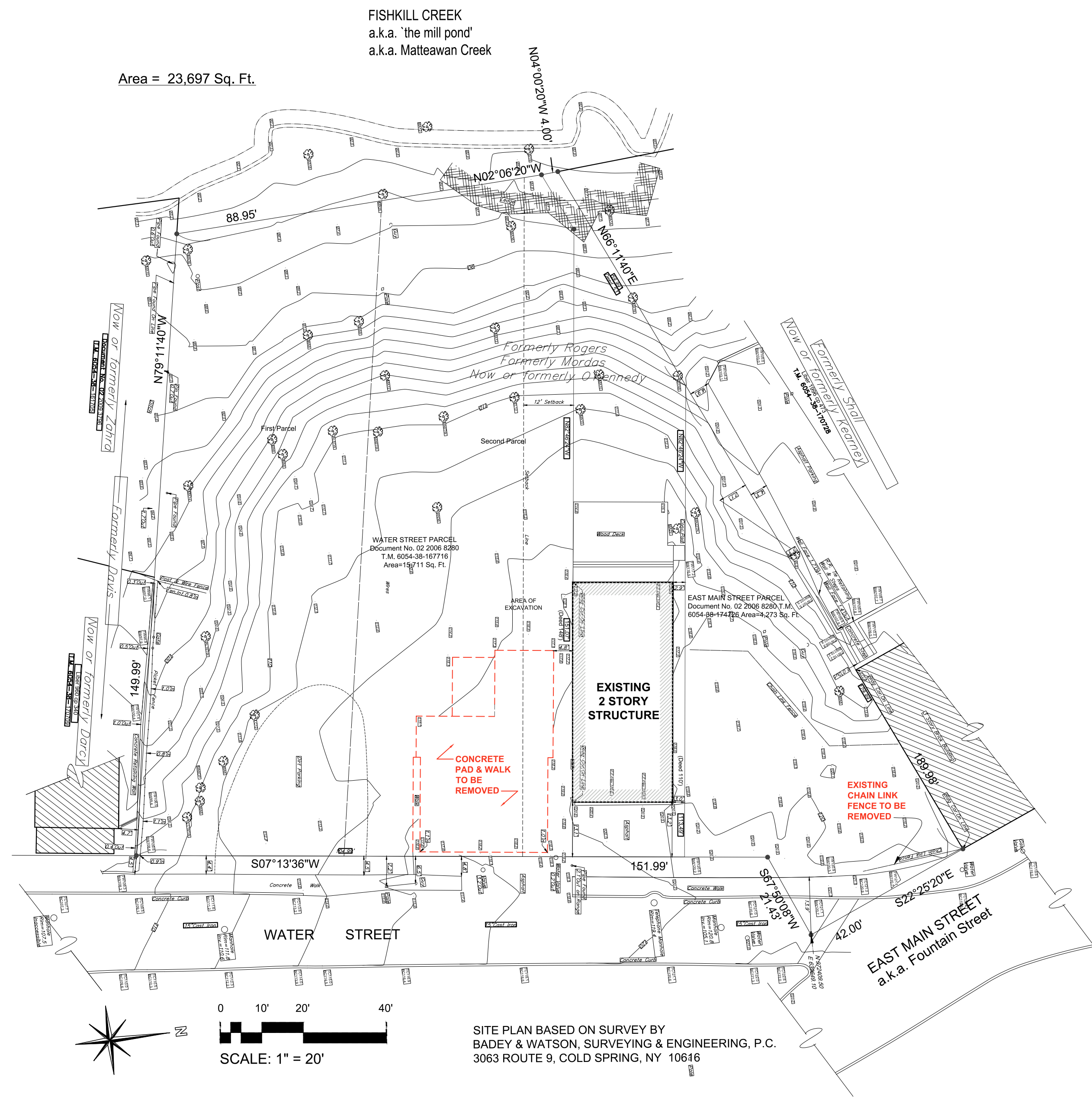
Site Demolition Plan Scale: 1" = 20'
