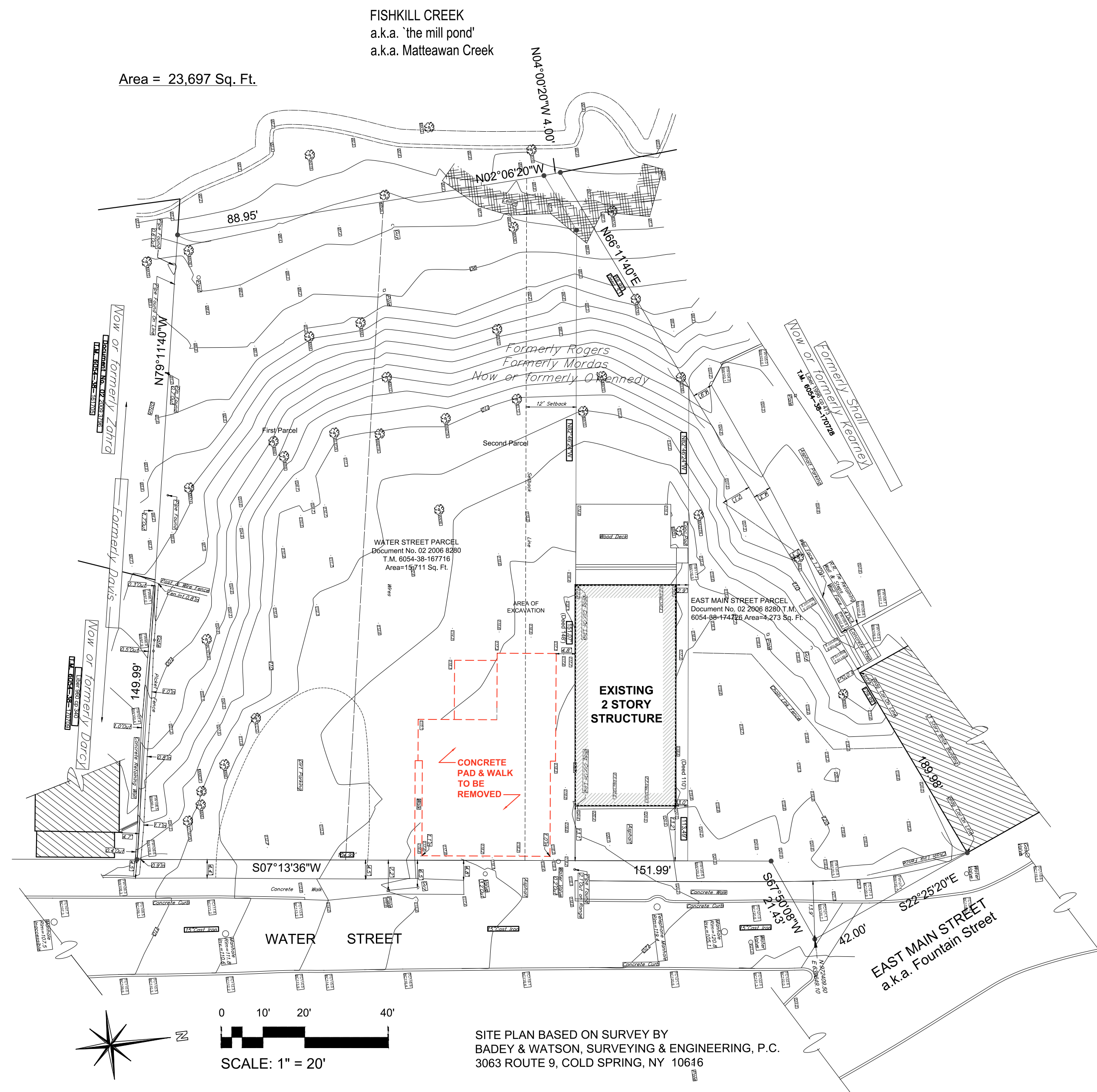
Site Demolition Plan Scale: 1" = 20'
