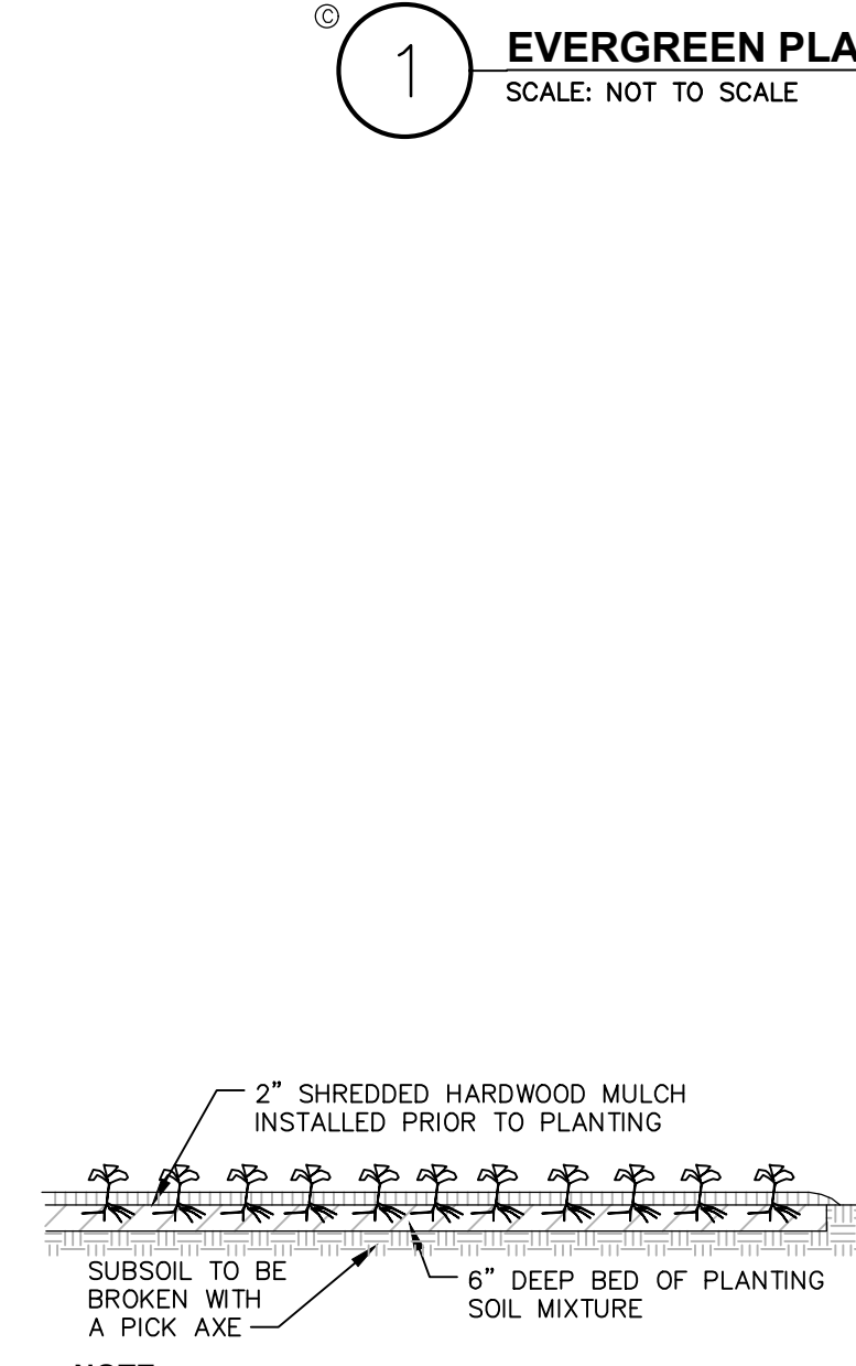
4 GROUND COVER/ANNUAL PLUG PLANTING SCALE: NOT TO SCALE LAST REVISED:
