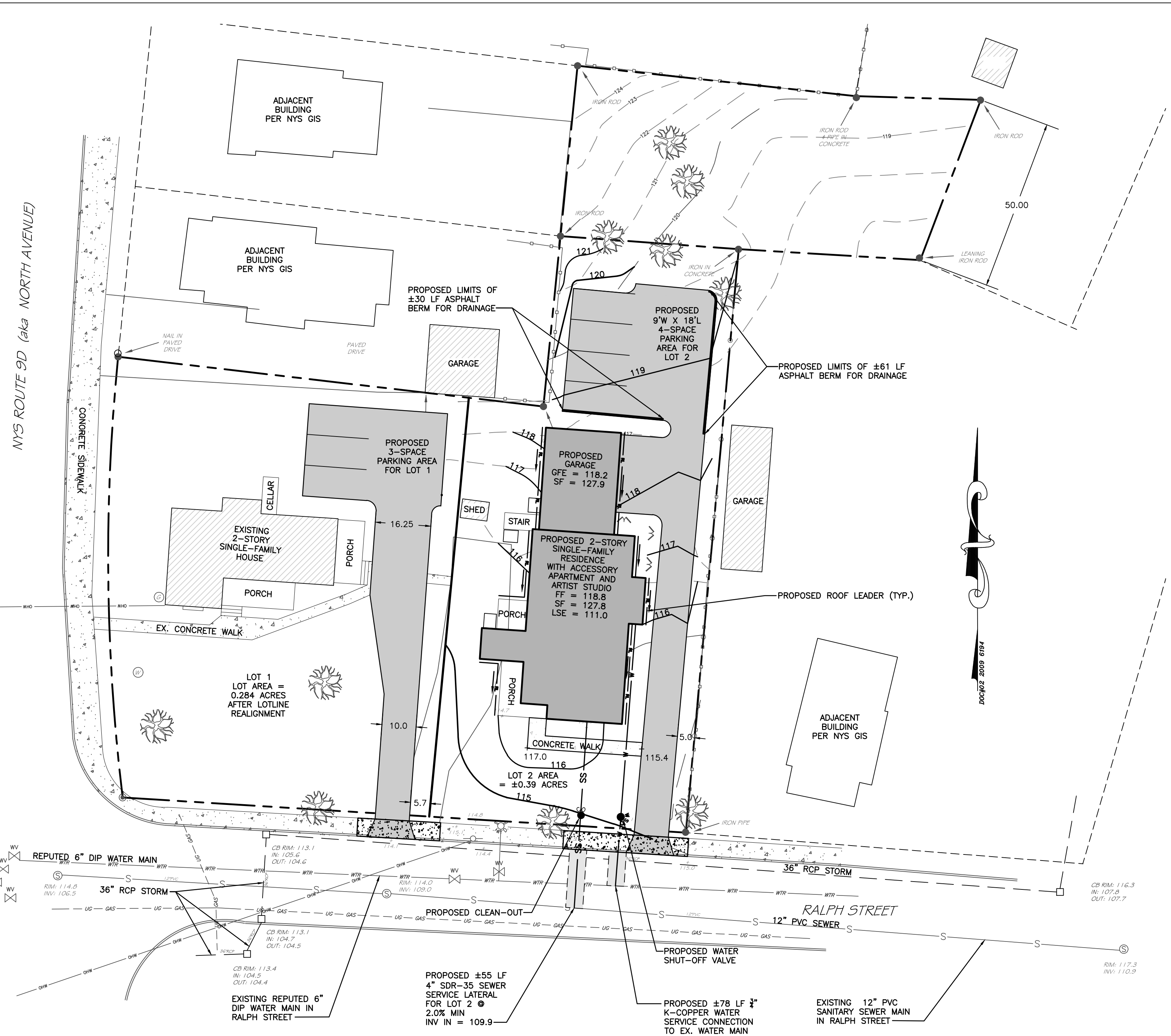
GRADING AND UTILITY PLAN SCALE: 1" = 20' GRAPHIC SCALE
