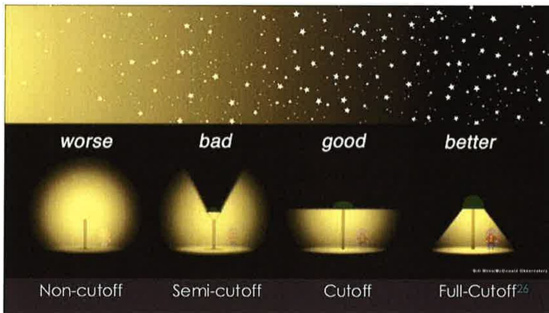
This illustrates the importance of full-cutoff fixtures. [Image credit: Bill Wren, McDonald Observatory]
