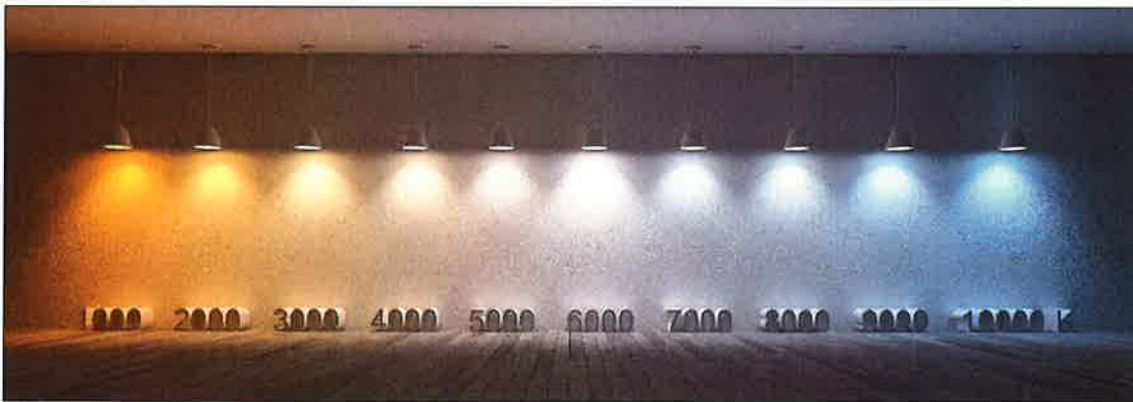
The range of colors shown here are pegged to their temperature, or K value, illuminated beneath each lamp. A standard incandescent bulb would fall around 2,700K – 3,000K. [Image credit: The Lighting Practice]
