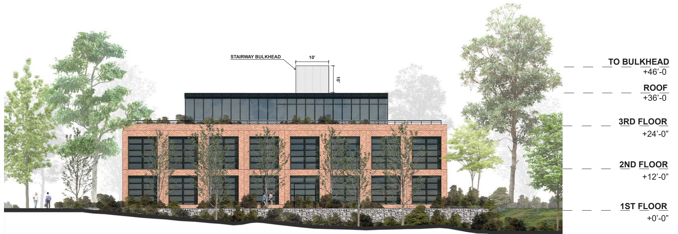
EAST ELEVATION BLDG 100
