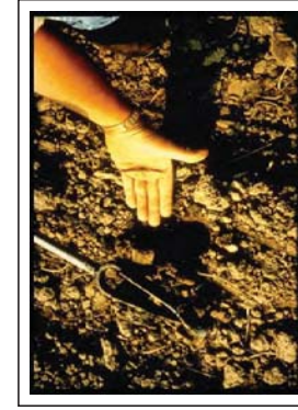
Fig. 5. Augered from a depth of 19 inches below the surface of the replaced topsoil, this subsoil sample was hand rolled to a 1/8-inch diameter. The test shows the soil at this site stretches out too far without crumbling; it indicates the material is in a plastic state of consistency, too wet for final decompaction (deep subsoiling) at this time.
