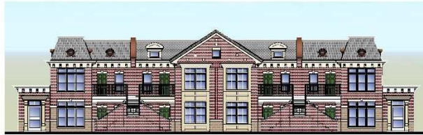
WEST ELEVATION - BUILDINGS 200 & 400 SCALE: 1/8" = 1'-0"
