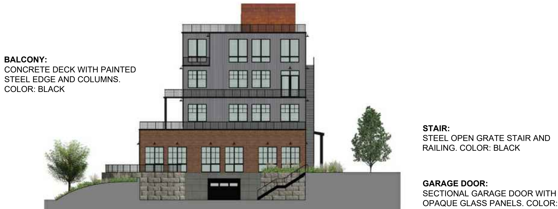
Elevation: North (South Similar) 1/8" = 1'-0"
