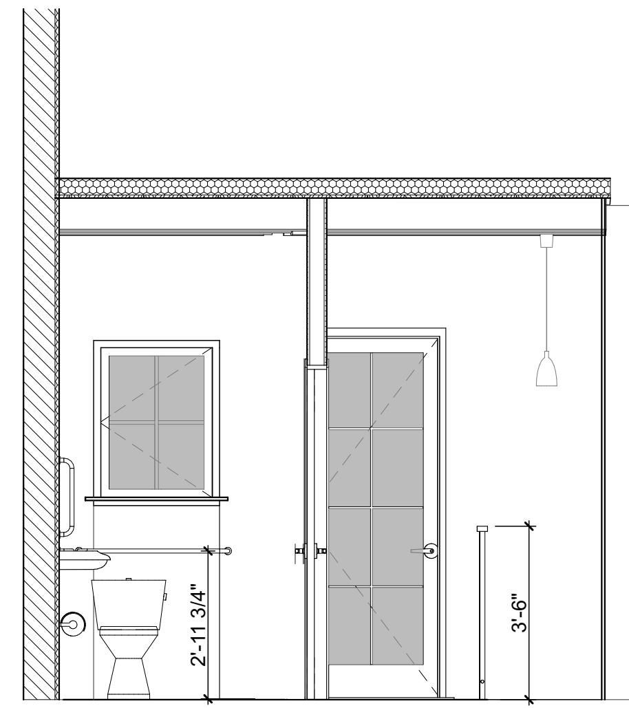
2 INTERIOR ELEVATION - ADA TOILET & HALL SCALE: 3/8" = 1'-0"
