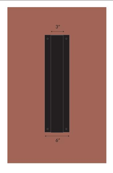
Anchored to masonry with (4) painted stainless lag bolts with lead shields.
