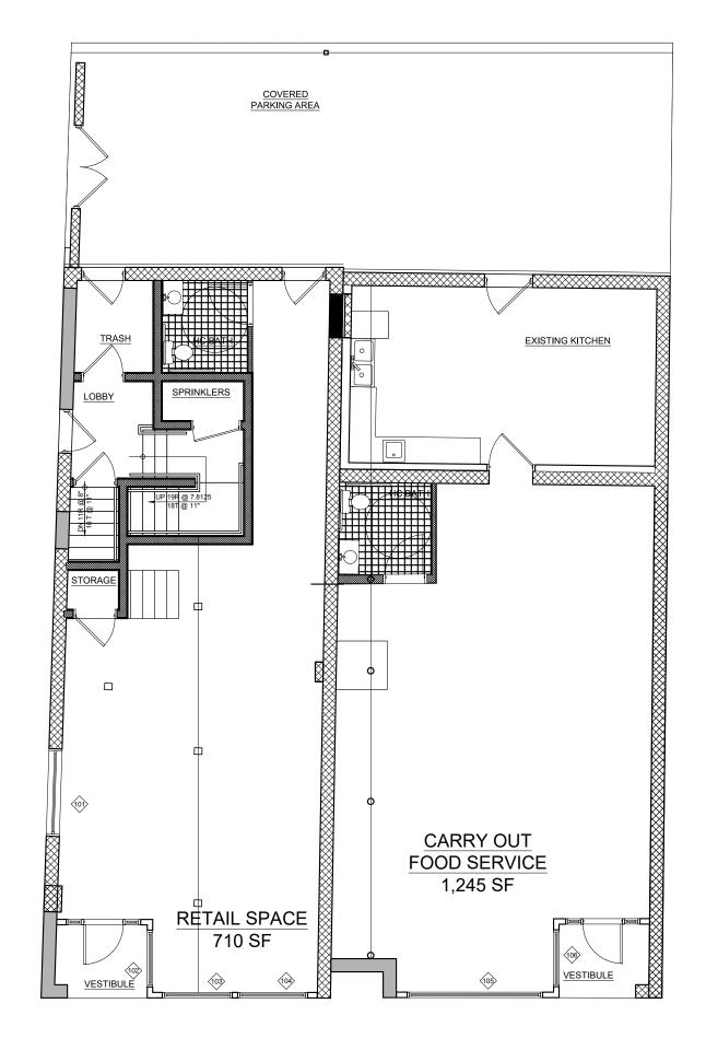
**1st Floor Plan** Scale:  $\frac{1}{8}$ " = 1'-0"
