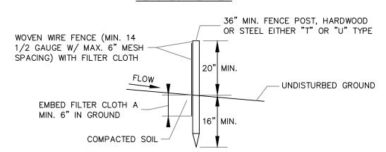
SECTION VIEW 1. FILTER CLOTH TO BE FASTENED SECURELY TO WOVEN WIRE FENCE WITH TIES
