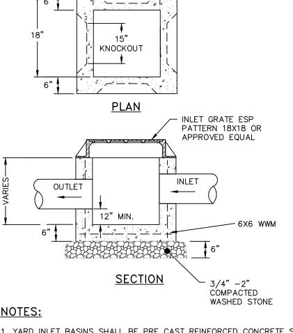
1. YARD INLET BASINS SHALL BE PRE CAST REINFORCED CONCRETE SHALL HAVE A MINIMUM 28-DAY COMPRESSIVE STRENGTH OF 4,000 PSI AND SHALL BE IN CONFORMANCE WITH ASTM 478-68. WALLS AND BASE SHALL BE ONE PIECE CONSTRUCTION. YARD INLET BASIN SHOWN BY EXPANDED SUPPLY PRODUCTS (ESP), 3330 ROUTE 9, COLD SPRING, NY (845) 265-3771. 2. BACKFILL USING SELECT MATERIAL, COMPACTED IN 6" LIFTS.
