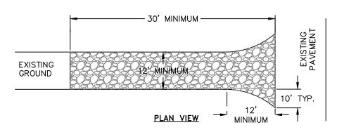
1) STONE SIZE - USE 1-4 INCH STONE, OR RECLAIMED OR RECYCLED CONCRETE EQUIVALENT.
