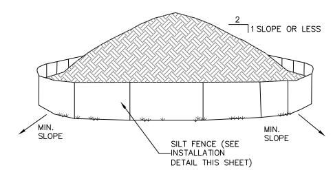
1. AREA CHOSEN FOR STOCKPILING OPERATIONS SHALL BE DRY AND 2. EACH PILE SHALL BE SURROUNDED WITH SILT FENCING, THEN STABILIZED WITH VEGETATION OR COVERED.
