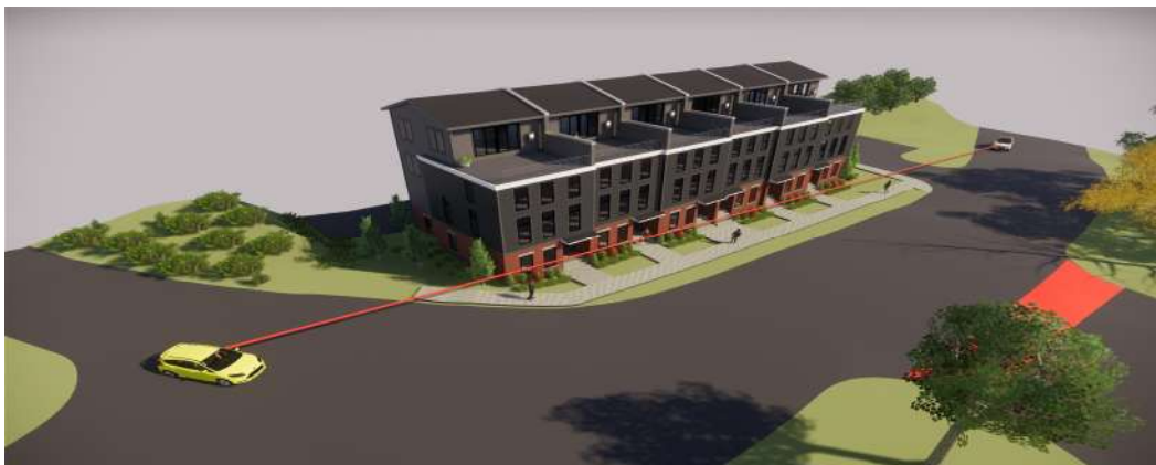
Figure 3: View of proposed sight distance conditions to the left for vehicles exiting Ferry Street. As vehicles move forward toward the through street sight distance is not obstructed by the proposed building. Additionally, the sight line at the front of the proposed building is improved with the removal of the existing concrete barrier blocks
