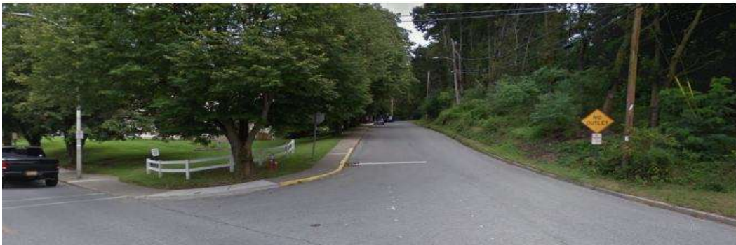
Figure 2: View of existing sight distance conditions to the right for vehicles exiting Ferry Street currently limited by the existing light pole, street trees, hydrant, and fence
