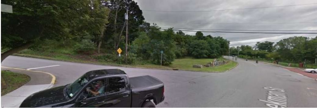
Figure 1: View of existing sight distance conditions to the left for vehicles exiting Ferry Street currently limited by the existing topography, vegetation, and the existing concrete barrier blocks
